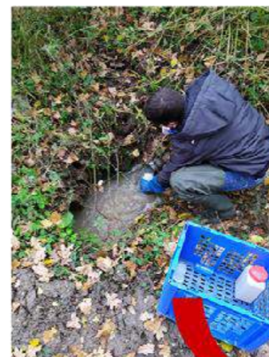
Drain Mr HEUSELE – PASSAGE A 10h50- DEBIT =4.3 l/s
