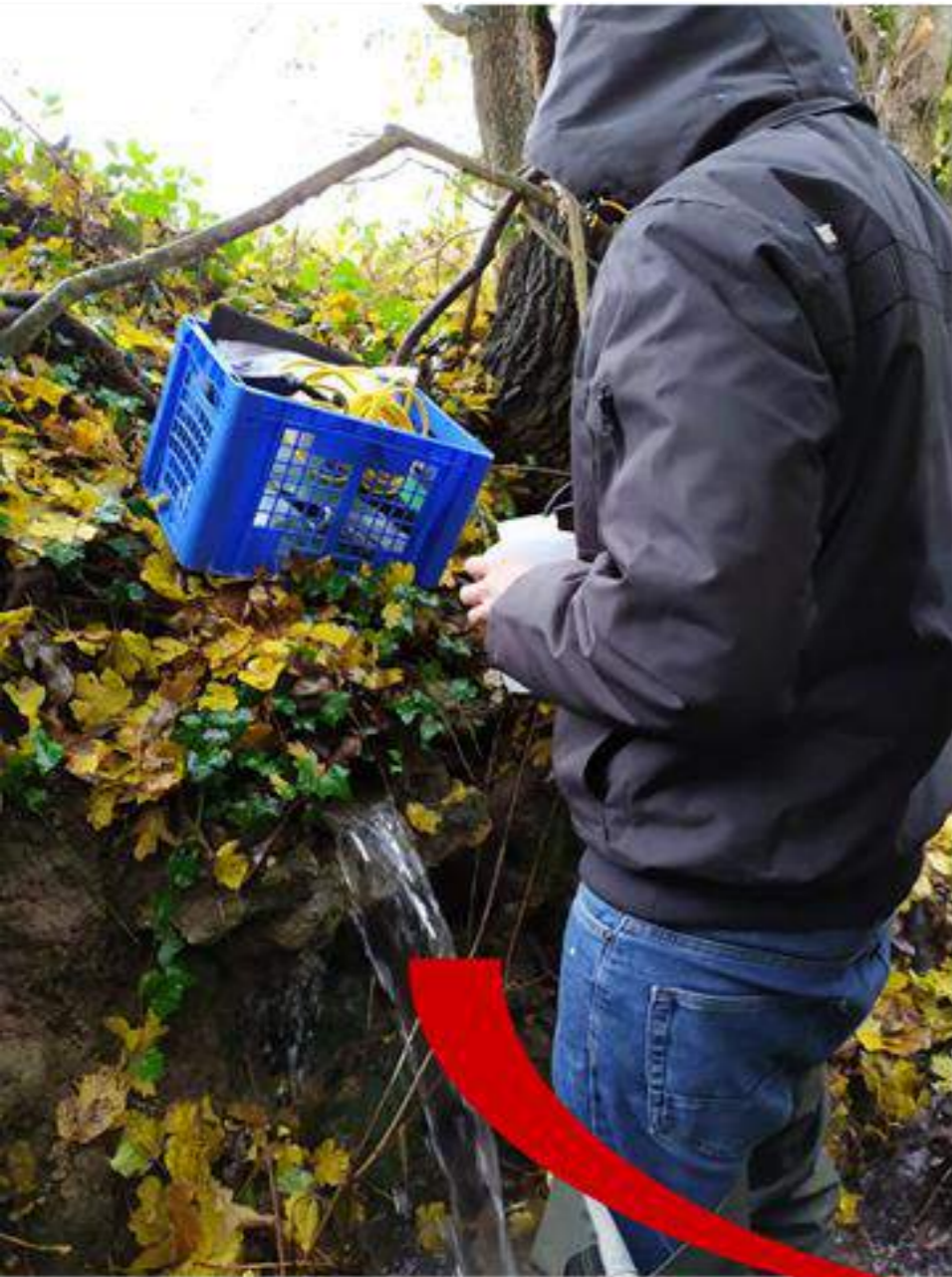
Drain Mr GILLOOTS – PASSAGE A 10h10- DEBIT =0.8 l/s
